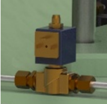
Fig 1. Solenoid valve for overspeed shutdown
