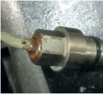
Fig. 2a: Defective feedback sensor
