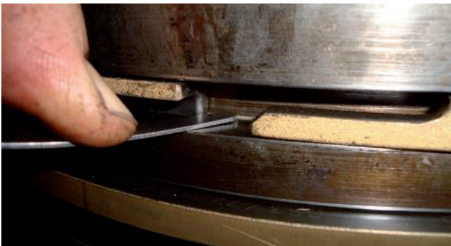
Fig. 2: Excessive ring groove wear and gap in the gas-tight lock
