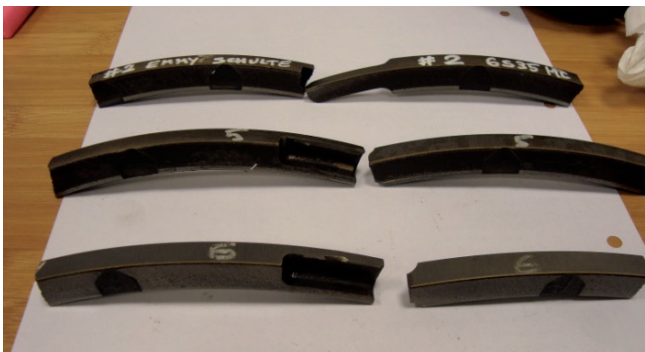
Fig. 3: Excessive ring groove wear and missing contact between groove and ring resulted in worn-out piston rings with gaps in the gas-tight lock
