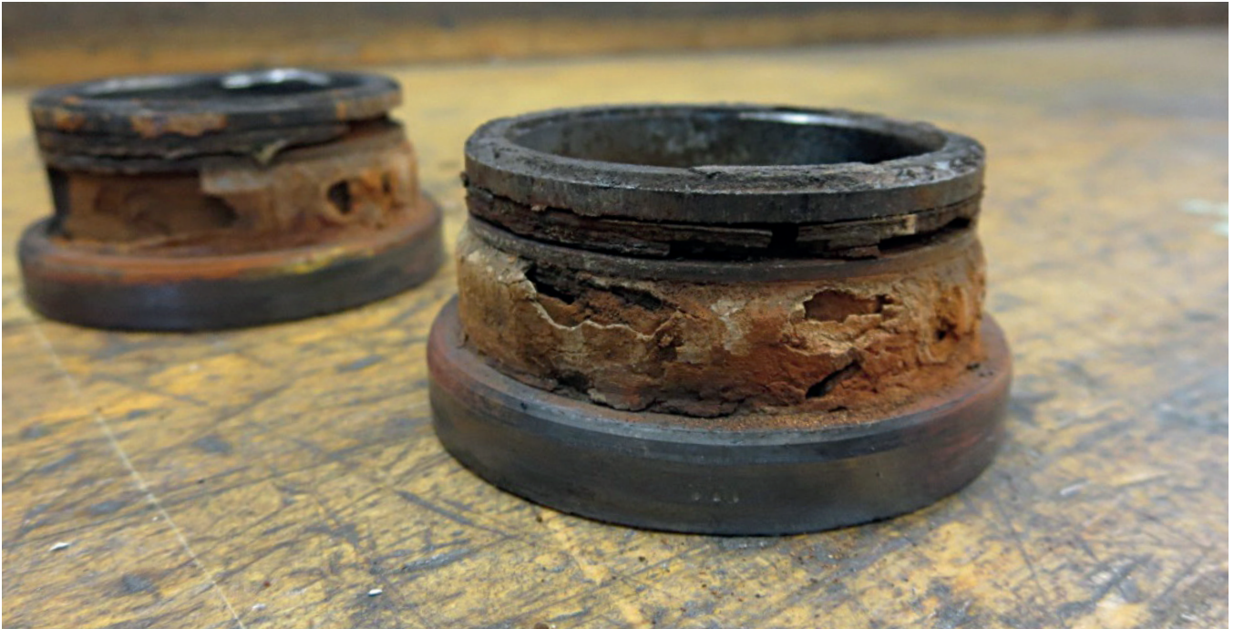
Fig. 1: Rust and limescale fill up the cooling space of the exhaust valve seat ring, and the O-ring has become hard and brittle
