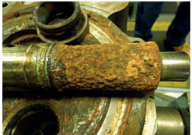
Fig. 2: Layers of rust and lime scale reduces the transfer of heat from the fuel injection nozzle
