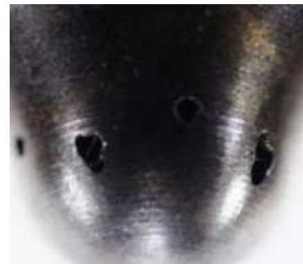
Excessive wear of fuel injector (nozzle holes)
