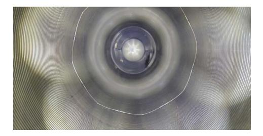
Recently, MAN Diesel & Turbo introduced the possibility of measuring all installed liners by the use of online laser-based equipment, a so-called VAK. This system does not require lifting of cylinder covers or exhaust valves, but only the removal of one cylinder cover mounted fuel oil valve.
