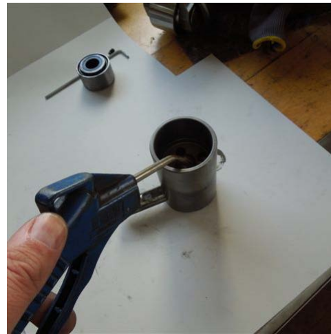
Clean the roller guide by air and diesel oil if required.
