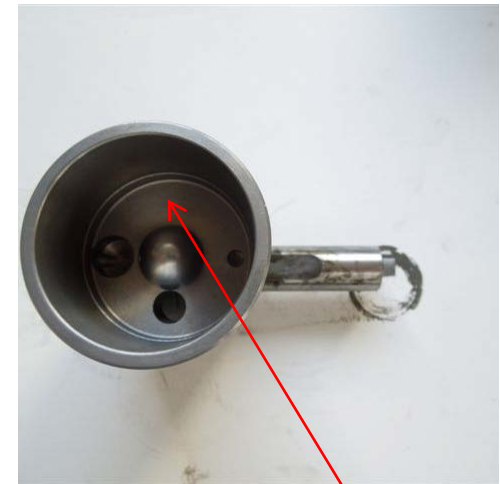
Punch mark opposite side of the existing drain hole
