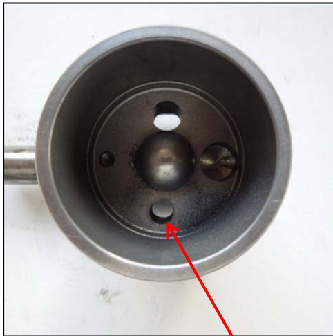
New drain hole
