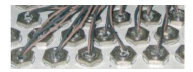
• Make sure that the shield is installed correctly in the cable union to avoid electromagnetic compatibility
