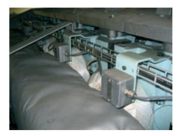
Dismantle all sensors and junction boxes for both cylinder and turbocharger
