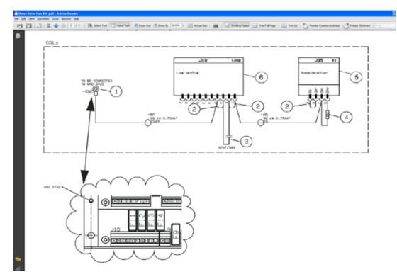
Figure 1: An illustration of the hardware installation part of the "Noise detect" functionality. The illustration is taken from S906-0048, issued by MAN Diesel & Turbo. '1' is a cable shoe connected to a ground stud, '3' is a capacitor (47nF/50V) and '4' is a 2k2Ω resistor.
