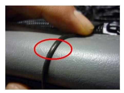
Figure 22: The resulting loss of insulation. Giving rise to the electrical noise.
