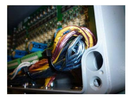
Figure 9: Close-up of the end of the wire bundle, indicating how it can chafe against the box.
