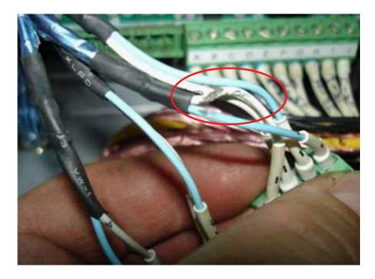
Figure 11: Additional chafing of the wires close to the plugs (red circle).
