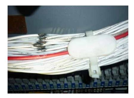
Figure 18: Close-up of the place where the insulation was worn off. Note this was on the rear side of the wires, therefore it was necessary to twist the bundle before the failure could be seen.
