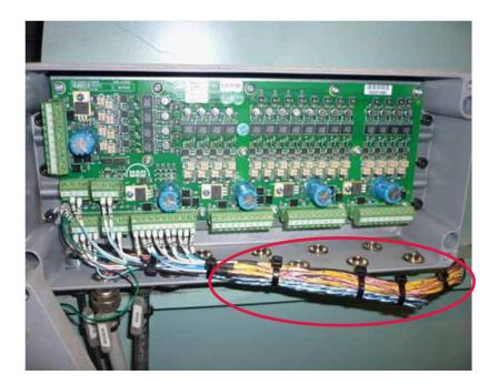
Figure 8: The open TSA box. Clearly showing the long, unsupported coil of wires (red oval).
