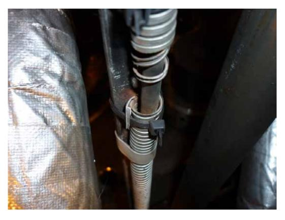
Figure 16: Wire protection broken; giving rise to sharp edges that can destroy the insulation of the wire.
