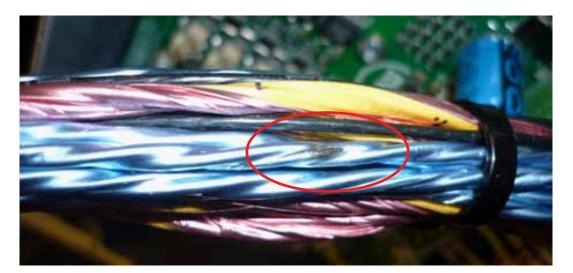
Figure 10: After the wire bundle has been opened up, the failure in the insulation can be seen (red circle).
