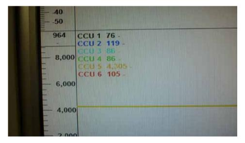
Figure 3: Example of very clear indication of an intermittent low insulation on CCU-5. This fault was located to be chamfered wires inside a MTBEV junction box.
