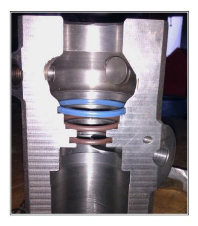
The sealing ring must be mounted with the spring facing upwards. Press the sealing by hands until it "clicks" down.
