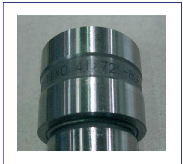
Fig 4 Nozzle element with specification and IMO number
