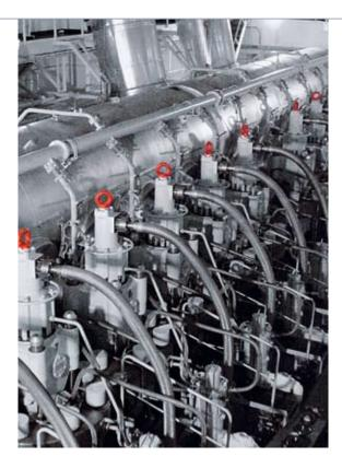
This 4-day course covers the MAN B&W electronically controlled small bore engine with camshaft operated exhaust valves – the ME-B engine. It concentrates on the electronic and hydraulic control systems. Only mechanical/structural parts differing from MC engine specification are covered, e.g. camshaft, fuel oil pressure booster. Parts shared with the MC engine are covered in our general MC engine training course.
