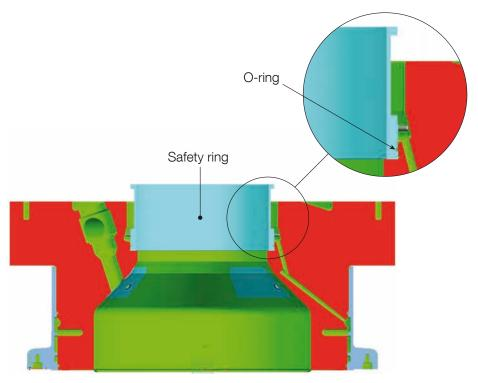
Fig. 1: Safety ring mounted in exhaust valve hole
