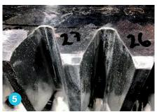
Onshore or offshore, our team of specialists will use a combination of machining, welding and polishing to recover the damaged area tooth by tooth. Depending on the damage, the area or tooth will be machined to achieve a clean surface, new material will be added by welding and the final shape and surface of the tooth achieved by polishing. Finally, thorough measurements of each tooth assures that all specifications are met making the wind turbine fully operational again.
