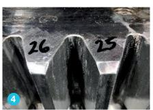
When for different reasons a yaw ring tooth or series of teeth has been worn or damaged, the fastest and most cost-effective way of bringing the yaw ring back to original specifications is on-site recovery.
