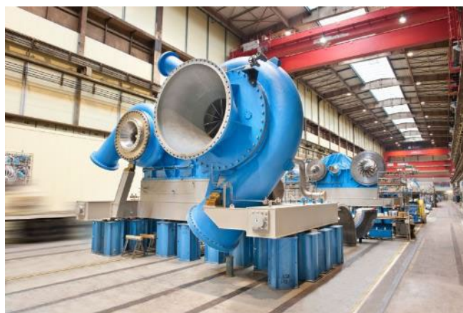
RG integrally geared type compressors by MAN Energy Solutions
