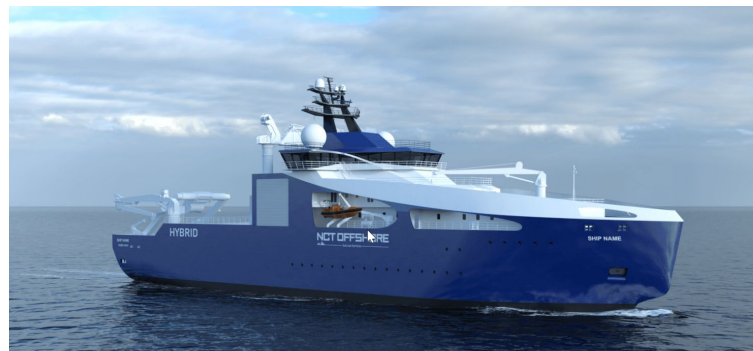
Graphical rendering of the newbuilding cable-laying vessel (picture courtesy VARD). The 95-metre CLV has single-cabin accommodation for 60 persons and will be capable of providing turn-key array cable T&I scopes of work for large-scale, offshore renewable projects
