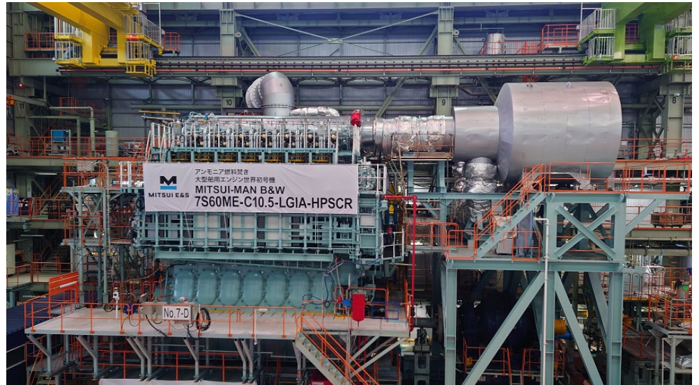
The 7S60ME-LGIA ammonia dual-fuel prototype engine pictured at the Tamano Factory (picture courtesy MITSUI E&S)
