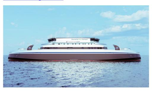
Graphical rendering of the newbuilding RoPax (courtesy Norwegian Ship Design). The new ferries will be about 120 m long with capacity for 120 cars and 599 passengers. They will serve a close to 100 km open ocean crossing above the Arctic Circle that is considered Norway's most challenging ferry crossing
