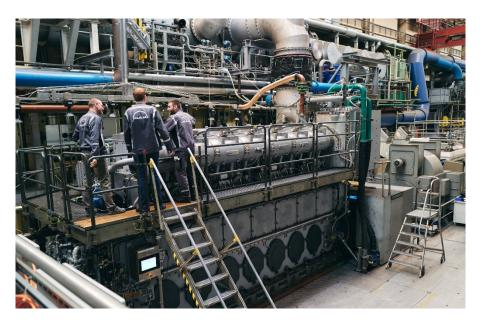
The conversion package for the 51/60R-DF-M has been tested intensively at the MAN Energy Solutions test bed in Augsburg, Germany since summer 2024. (Copyright: Stefan Hobmaier)
