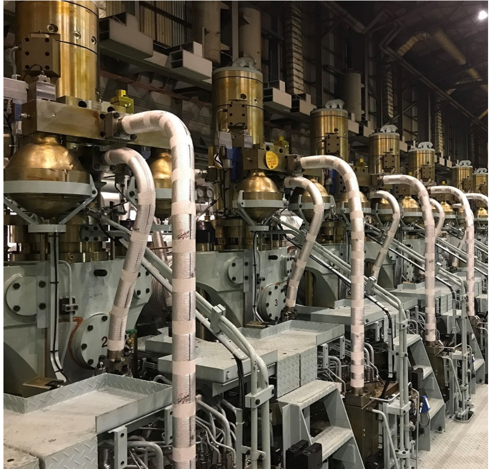
The MAN B&W ME-GI engine
