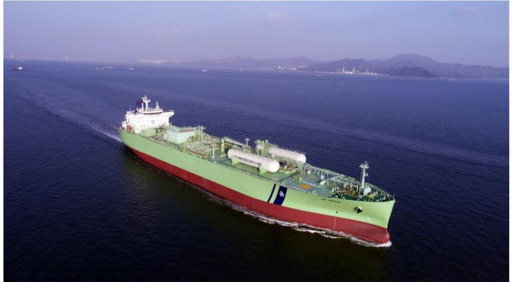
*The 'BW Gemini', a VLGC from the BW LPG fleet, has had its MAN B&W 6G60ME-C9.2 main engine retrofitted to an MAN B&W 6G60ME-C9.5-LGIP dual-fuel type, capable of operating on fuel oil and LPG. The conversion is the first of 15 for a series of LPG carriers owned by BW LPG (picture courtesy BW LPG)*
