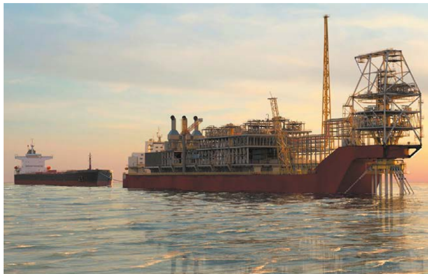
Illustration of the FPSO (floating production storage and offloading) unit for the Sangomar gas field development. – Courtesy of MODEC
