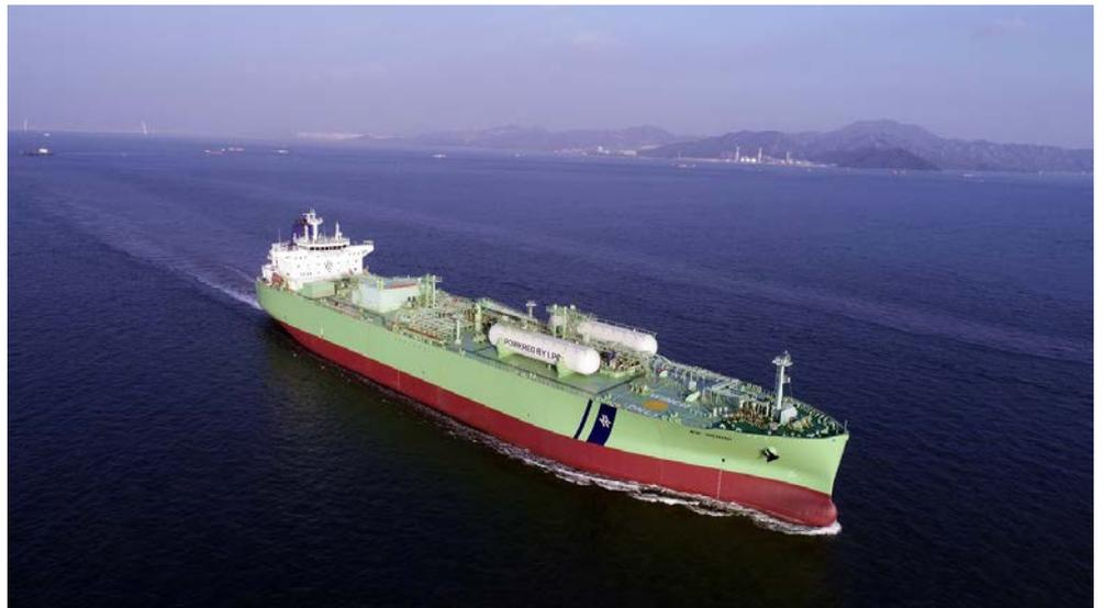
*The ‘BW Gemini’, a VLGC from the BW LPG fleet, has had its MAN B&W 6G60ME-C9.2 main engine retrofited to an MAN B&W 6G60ME- LGIP dual-fuel type, capable of operating on fuel oil and LPG. The conversion is the first of 12 for a series of LPG carriers owned by BW LPG (picture courtesy BW LPG)*
