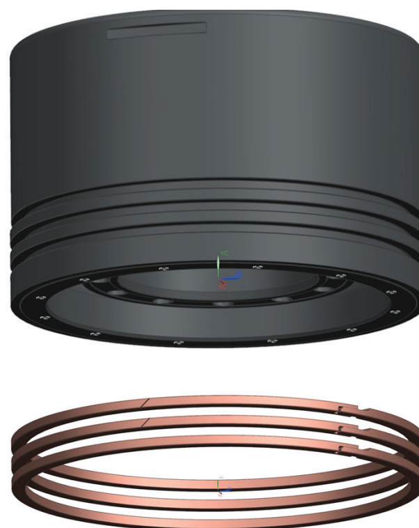
Fig. 2: New piston design
