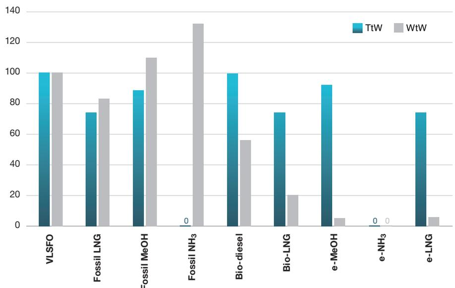
Fig. 10.4: Tank-to-wake and well-to-wake emissions of selected fuels relative to HFO [8], GWP100 of CH<sub>4</sub>=29.8 CO<sub>2</sub>eq
