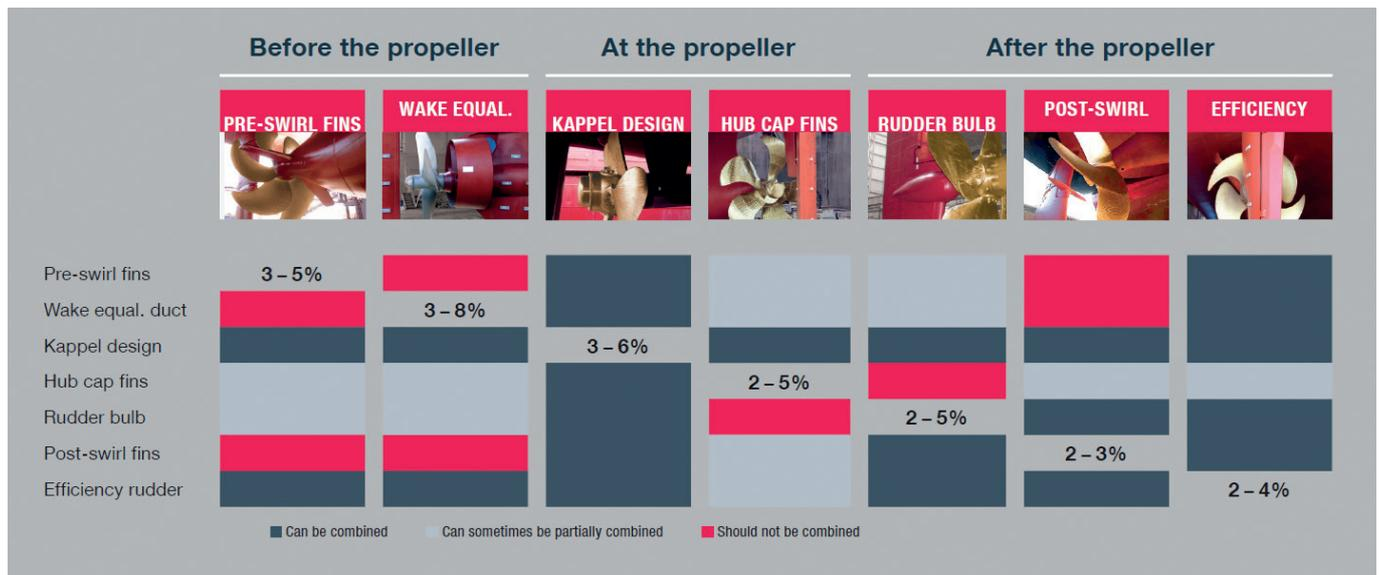
Fig. 10.18: Possibilities for combining energy saving devices, including individual saving potentials
