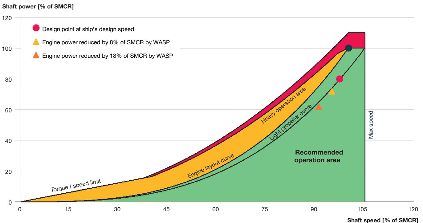
Fig. 10.17: Impact on the engine running with different thrusts provided by WASP. The contribution from a WASP system varies greatly depending on the wind direction and speed. Notice is given to somewhat lighter running of the propeller as the propeller does not need to deliver the full thrust.
