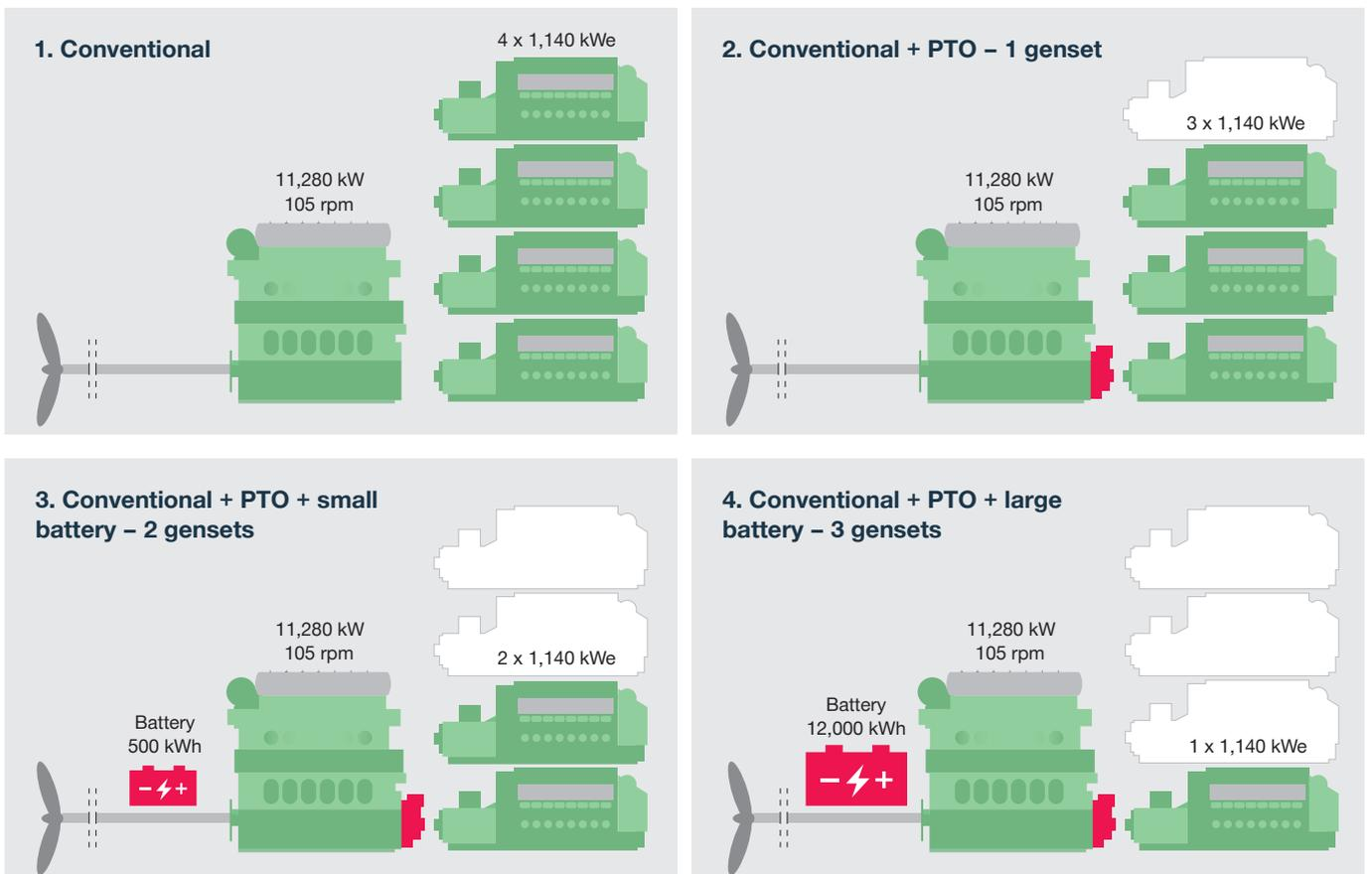
Fig. 10.10: Topology of four propulsion plants with various degrees of hybridisation for a container feeder
