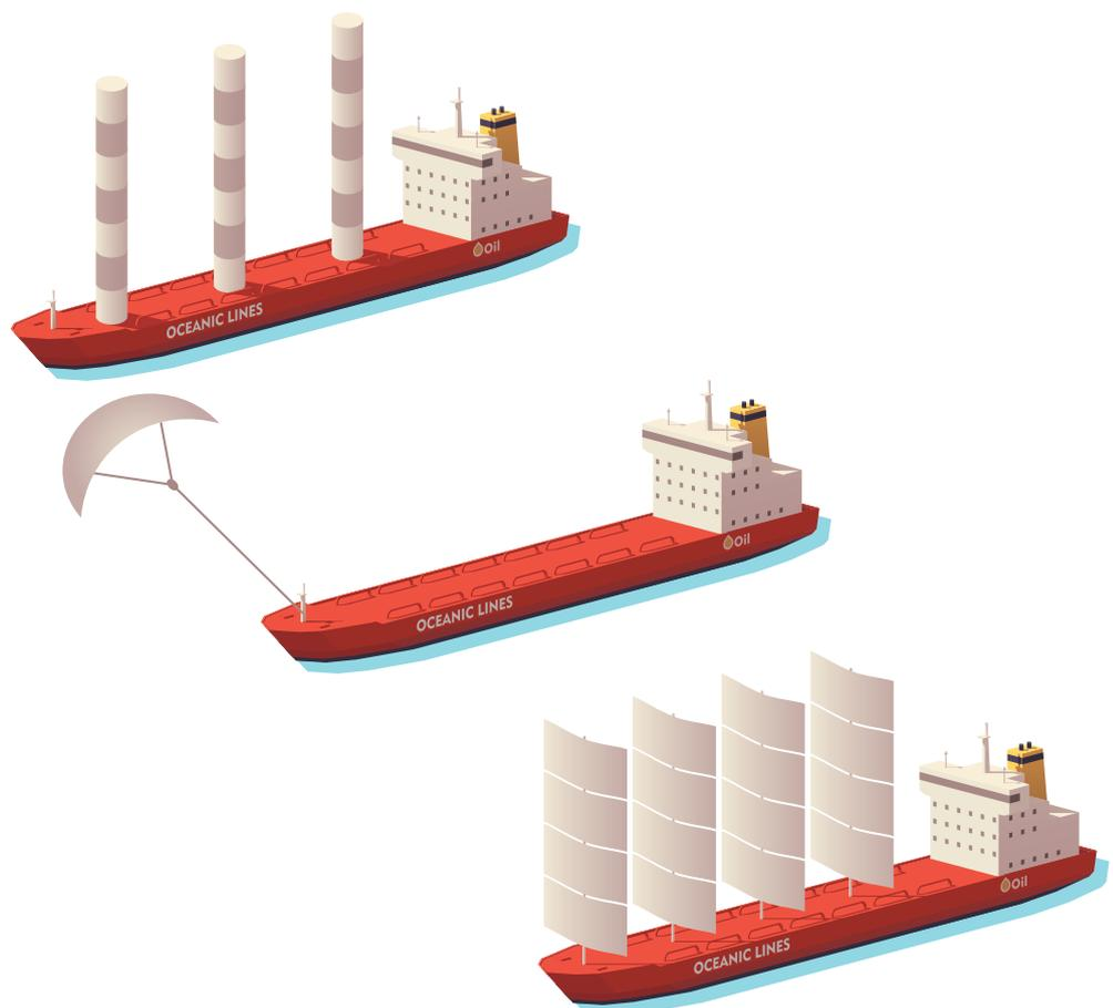
Fig. 10.16: Different types of wind-assisted propulsion technologies
