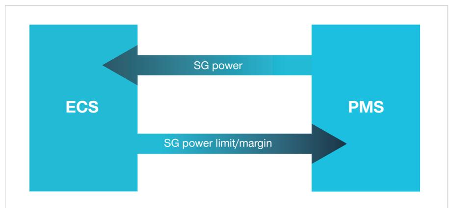
Fig. 10.7: Signals in interface option C
