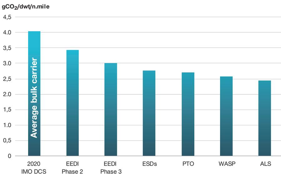
Fig. 10.19: Present CO<sub>2</sub> emissions [gCO<sub>2</sub>/dwt/nm] in IMO DCS for an average bulk carrier (84,000 dwt) together with the estimated impact of applying alternative technologies
