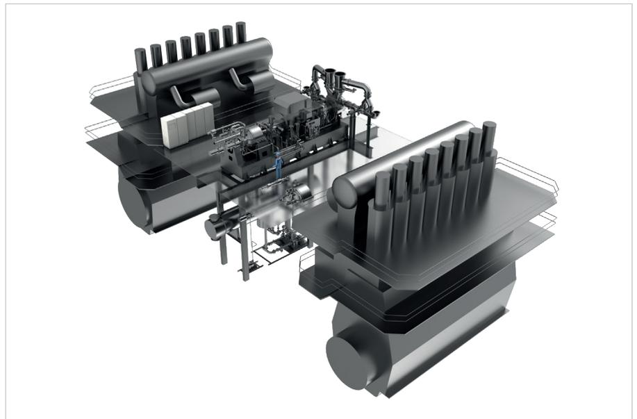
Fig. 10.13: WHRS with PTG + STG – design for twin-screw vessel
