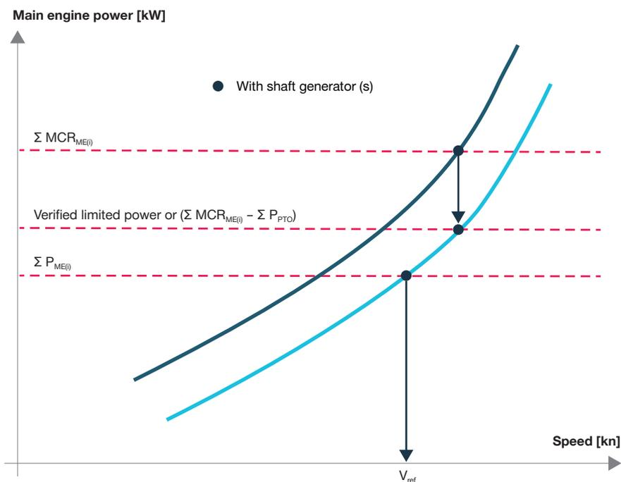
Fig. 10.8: Option 2 for inclusion of a PTO to the EEDI [10]
