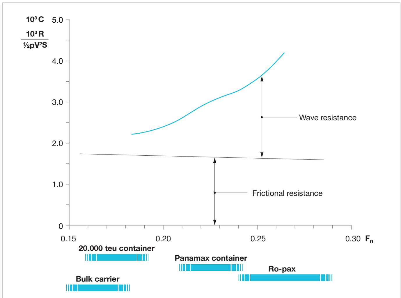
Fig. 10.14: Simplified illustration of the components of the total resistance as a function of the Froude number
