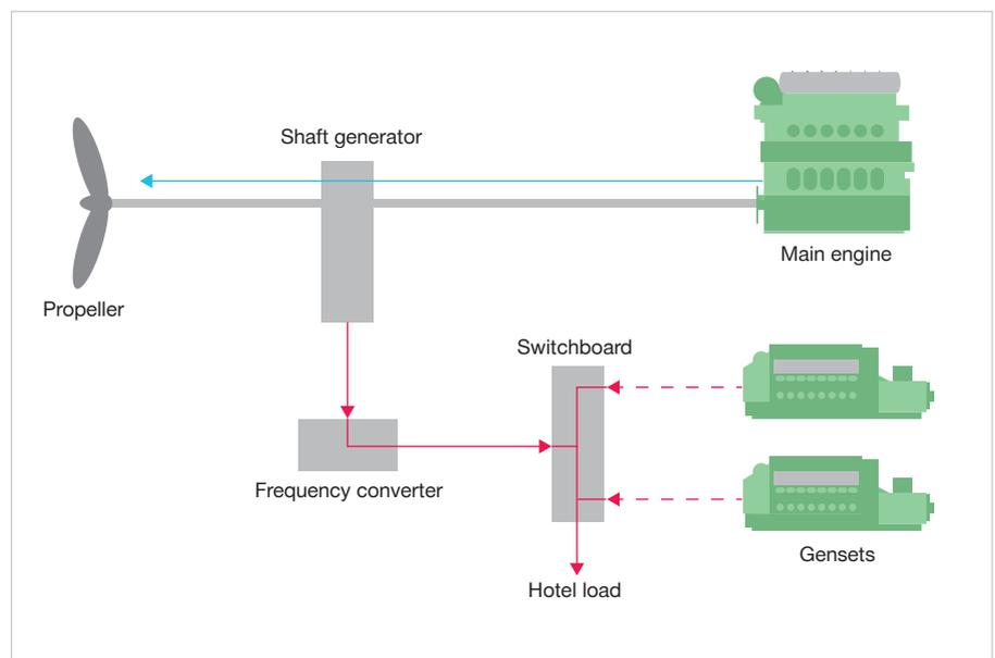
Fig. 10.6: Schematic illustration of a propulsion plant with shaft generator and integration with the electric power plant
