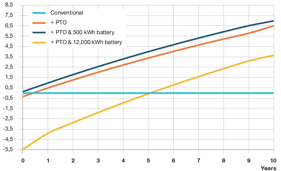
Fig. 10.12: Net present value of investing in PTO and batteries for a 1,700 teu feeder operating in Northern Europe
