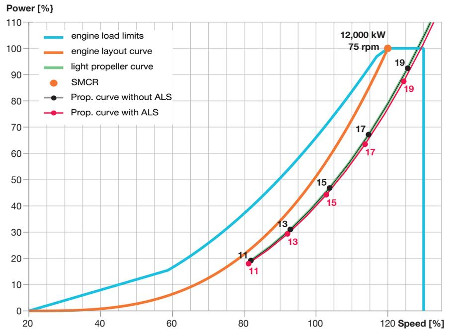
Fig. 10.15: Propeller curves with and without an active air lubrication system
