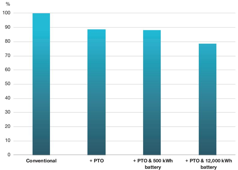
Fig. 10.11: Relative energy consumption by including a PTO and various battery capacities in the power generation system for a 1,700 teu container feeder
