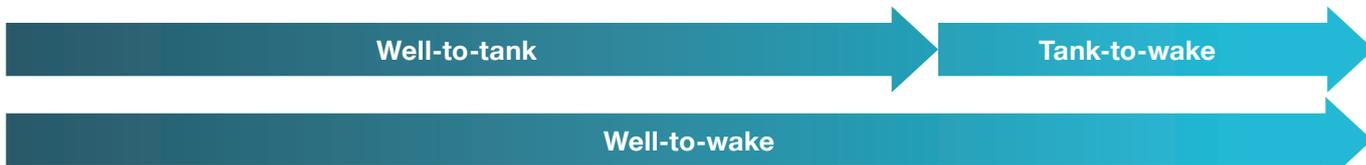
Fig. 10.3: Emission scopes: tank-to-wake, considering on-board emissions, well-to-wake, considering upstream emissions from the production of the fuel as well
