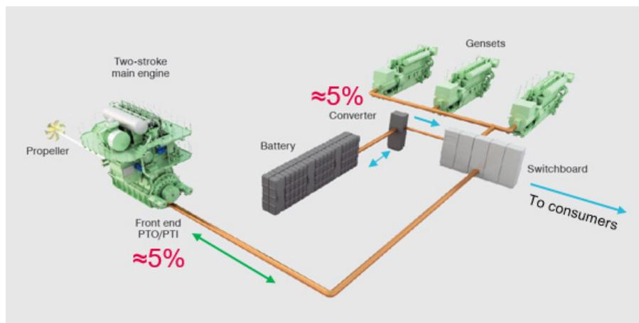
Fig. 10.9: Assumed losses in energy conversions for evaluating peak shaving of a diesel-mechanic propulsion plant
