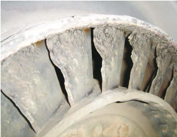
Damaged nozzle vanes
