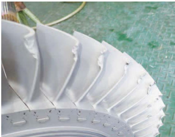
Damaged turbine blades
