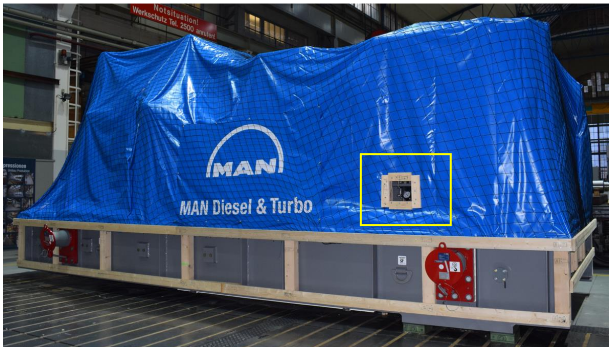
Figure 010: Pressure indicator and refill nozzle, access on the skid
