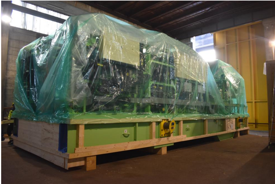
Figure 008: Skid completely covered with VCI foil
