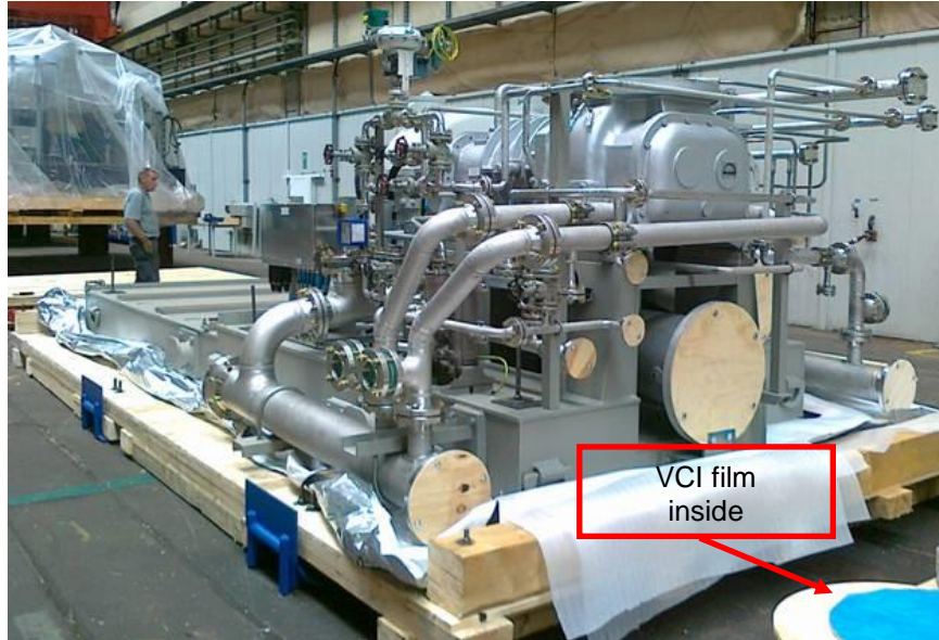
Skid with pipes closed with wooden covers
