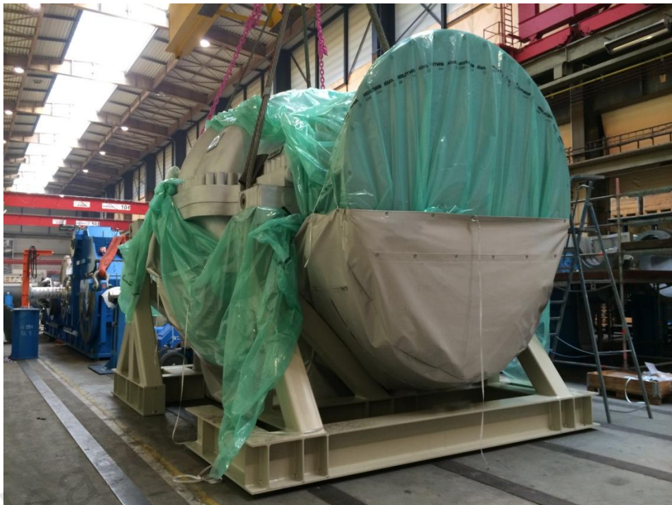
Axial compressor during the packaging (green: VCI film, gray: industrial tarpaulin)
