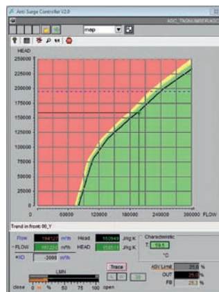
Real time plotting of compressor data in HMI
