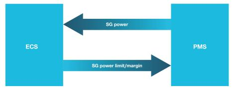
The ECS sends information to the PMS about the power margin to engine overload, thereby enabling the PMS to adjust the PTO load and avoid engine overload. The PMS returns information about the current PTO load to the ECS.
