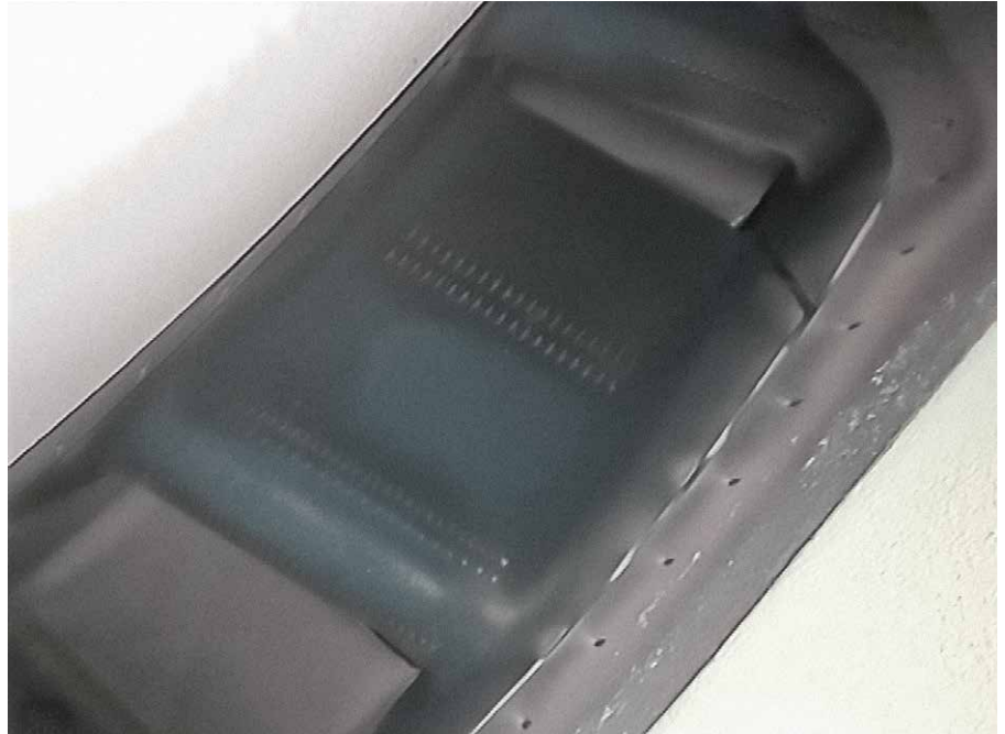
Picture 7: MGT6000 turbine inlet section after 37'100 equivalent operating hours (picture of borescope inspection on February 20, 2021)
