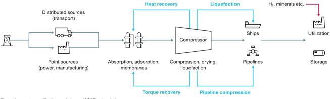
The carbon capture, utilization, and storage (CCUS) value chain
