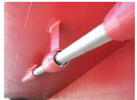
Shafting: Struts, bearings and an Inconel clad-welded tail shaft
