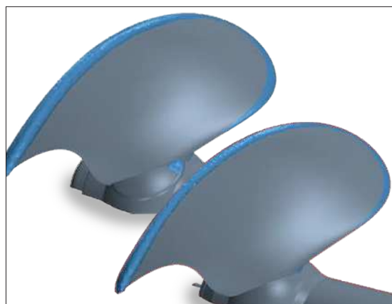
High blade loading simulation – reduced root cavitation below
