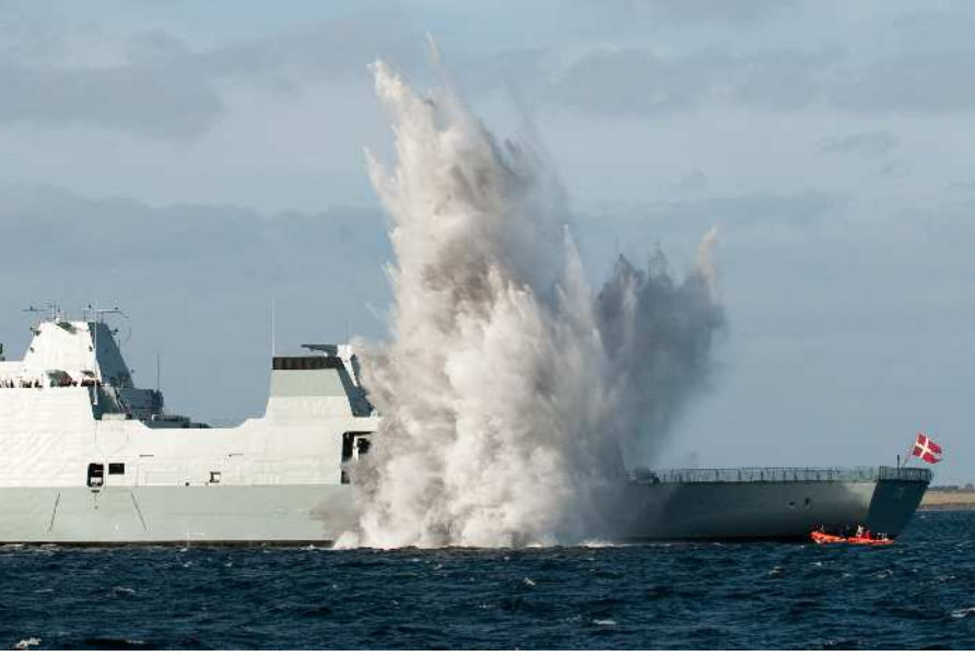
Full-scale shock testing – from underwater explosion
