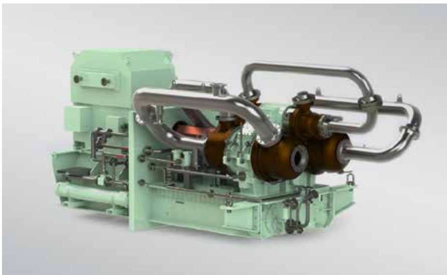
Fig. 15: BOG compressor from Cryostar (Courtesy of Cryostar)
