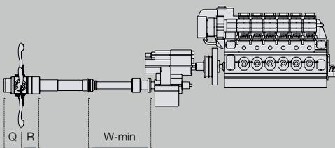
The standard 4-bladed propeller program is dimensioned according to Lloyd's Register No Ice.
