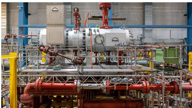
Heat pump unit on the test bed
