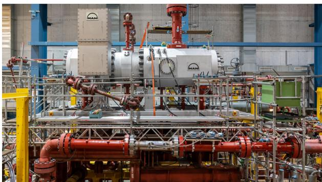
Heat pump unit on the test bed
