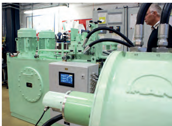
Factory test of oil distribution unit and hydraulic power unit
