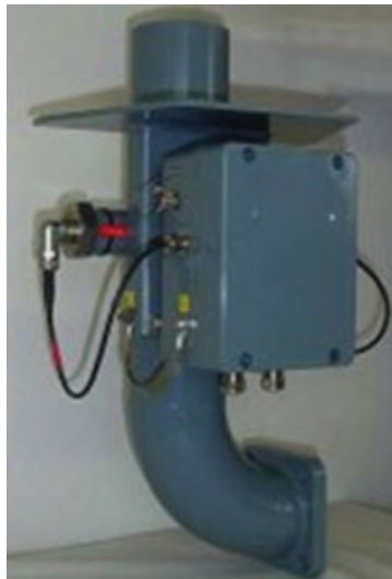
Figure 1: Oil mist detector.
