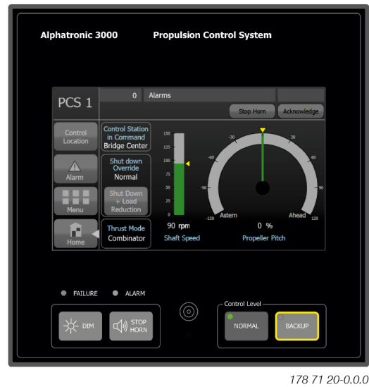
Fig. 5.18.10: Propulsion control panel – PCP – for CPP plants
